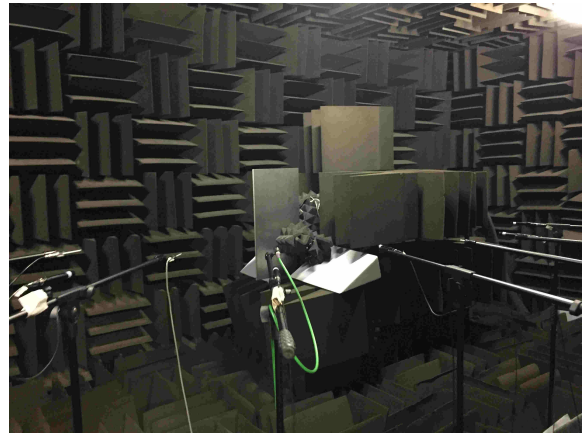
Fig. 2 The installed jet noise experiment setup: microphones are located at 50D to the jet nozzle center on the shielded side, with observer angle ranging from 30^\circ to 120^\circ to the jet centerline. The nozzle is behind the rectangular flat plate. The plate is then uninstalled and mounted on the other side of the jet nozzle to measure the noise spectra on the reflected side.
